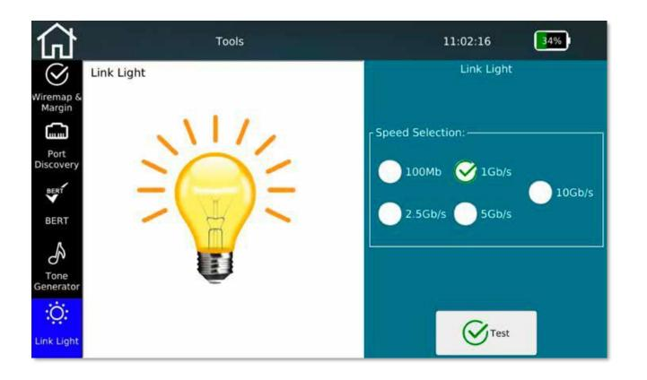
Accessed from the Tools menu, the Link Light function causes the link light on the switch to blink for easy port ID.
