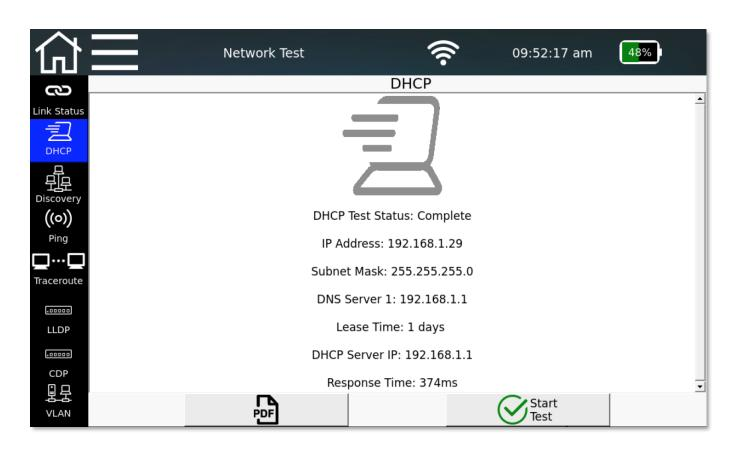
Verifies that DHCP is enabled and displays IP addresses for the server, gateway, Submask, DNS server and router.
