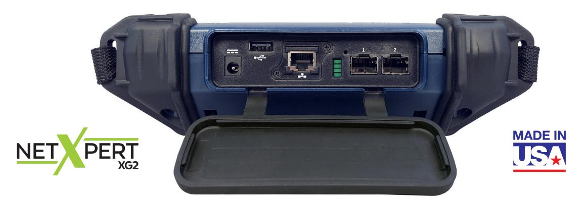
XG2 interface options include a field-replaceable RJ45 port, dual SFP+ ports, and a USB A port for easy use of thumb drives for report storage and transfer or even specialty networking dongles.
