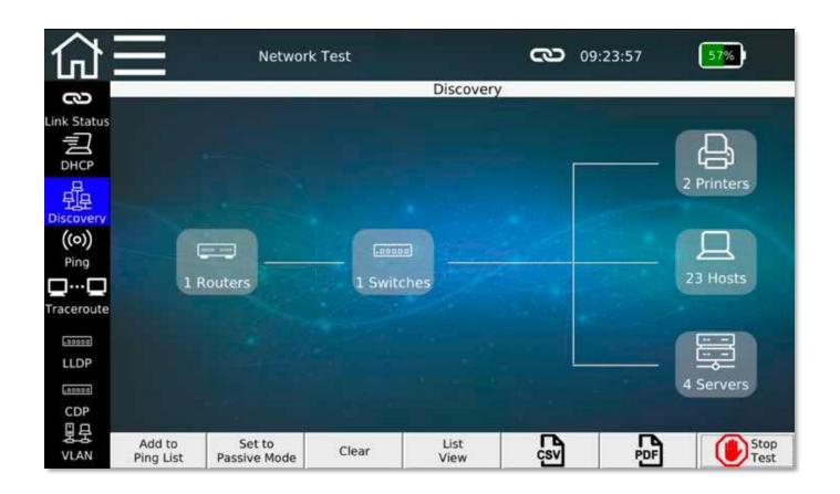
The Network Discovery Map provides a powerful overview of the entire submask and can also display the IP addresses of each attached device.
