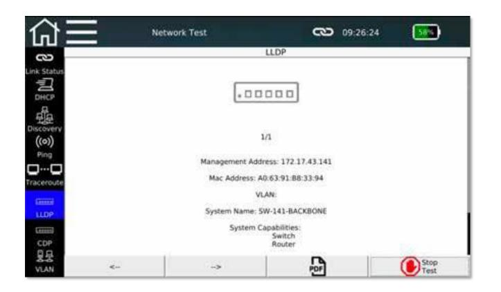
Detects Cisco Discovery Protocol (CDP) or Link Layer Discovery Protocol (LLDP) and displays information broadcast by the switch.
